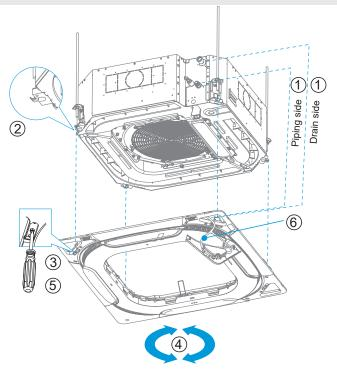
Suspend the decoration panel: Hang the two auxiliary hooks of the decoration panel onto the two hooks of the IDU's air guide ring. Then hang the four steel wire buckles for suspension onto the hooks at the four corners of the IDU, as indicated by the serial number ② in the figure. Note that the hooks are those hanging, protruded hooks.
