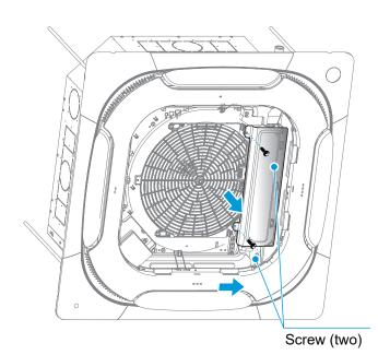
Remove the room temperature sensor for troubleshooting and repair.
