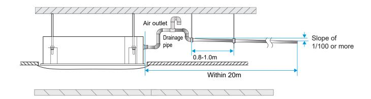
The end of the drainage pipe must be more than 50mm above the ground or from the base of the water discharge slot. In addition, do not submerge it in water. To discharge the condensed water directly into a ditch, the water discharge pipe must bend upwards to form a U-shaped water plug to stop odors from entering the room via the water discharge pipe.
