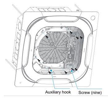
Replace the fan after removing the nuts at the center of the fan and the fan clip. Remove the nuts with flat washers and the fan clip at the position shown in the figure, and remove the centrifugal fan.
