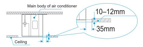
c. After the main body position and level are adjusted, tighten the nuts on the lifting bolts to secure the air conditioner.
