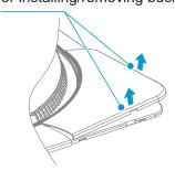
Loosen the locking screws at four corners and remove the hooks at four corners of the panel from the IDU. Take the auxiliary hooks of the panel from the air guide ring to remove the panel.
