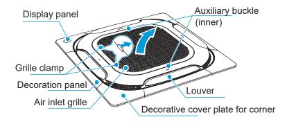
2 Raise the air inlet grille to about 45° and remove the grille.
