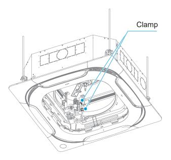
Remove the three motor bolts at the positions shown in the figure and remove the motor.
