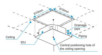
Determine the location of lifting bolts according to the lifting bolt hole at the four corners of the mounting cardboard.
