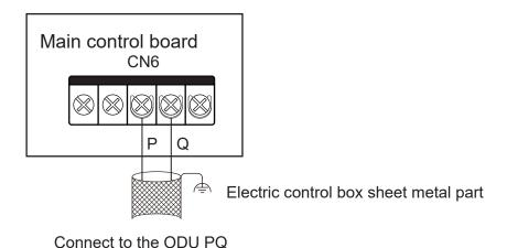
System: The maximum total length of the P/Q communication cable of the IDU and ODU can be up to 1200m, and can be connected in serial, as shown in the figure below:
