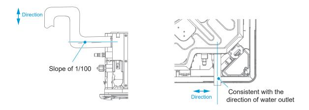
When connecting the drainage pipe, do not pull the drainage pipe forcefully, or it may become loose.
