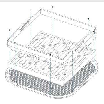
The G3 primary filter comes equipped with mesh screens. To replace the G3 and F6 filters, you lift one side and pull out the filter. To install a new filter, perform the step in the opposite direction.
