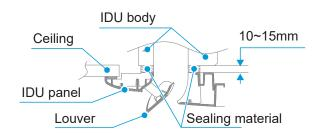
The ceiling shall have sufficient strength to ensure that the panel and the ceiling can be tightly fitted without gap. If the ceiling is not strong enough, add a stiffener. (See the figure below)
