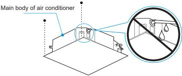
b. Adjust the position of the main body to ensure that the interval of the four sides of the ceiling is even, and the bottom surface of the main body should be recessed from the bottom surface of the ceiling by 10-12mm.
