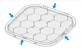
Pay attention to the direction of the G3 primary filter, including the airflow direction and mounting bracket direction. The wire mesh side is near the fan. The bracket should be placed as shown below, so that the filter can be pulled out easily. The G3 and F6 filters need mounting brackets, which are to be fixed at the air inlet grille using eight 3.9\*10 screws.
