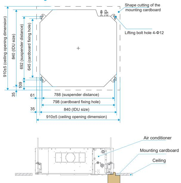
The mounting cardboard is used to adjust the distance between the air conditioner and the ceiling to ensure that the panel fits closely with the ceiling after installation.
