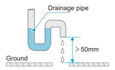
\* Connection method of the drainage pipe:
